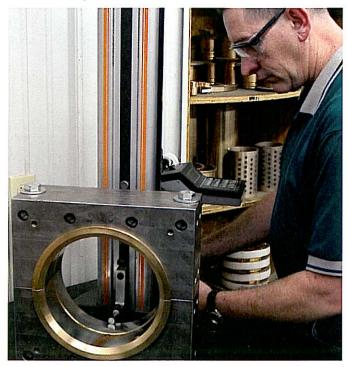
Final inspection is conducted with the bearing placed in precision ground fixtures to assure proper bearing clearance and crush.
