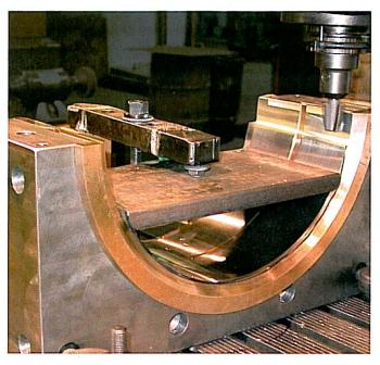
Precision ground fixtures are used to machine bearing crush. Bearing crush is the amount of the bearing shell that protrudes above the exact centerline of the main housing or connecting rod bore. Compressive force applied to the split line of a bearing conforms the bearing to the housing or connecting rod in which it is placed.
